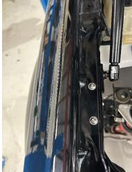
M6 Washers x 3 used for Spacer Between support Bracket and body on Right Hand Side. Install Right hand lower bracket to existing holes in front guard.
