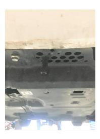
Step 13, Insert 8mm Drain hose (item13) into the holes on lower sump guard and trim hose as required.
