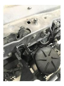
Step 12, Install Provent catch can assembly and mount to radiator support brace as shown
