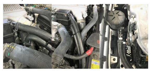
Step 14, Install 90 degree Breather hose (item9) with spring clamp 26/12 (item15) to air entry duct. Run hose next to radiator through foam holes and install to bottom port of the Provent with spring clamp 26/12 (item15). Hose may need trimming for perfect fit.
