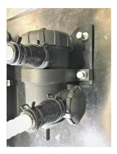
Step 4, Assemble Provent catch can to bracket using hardware shown.
