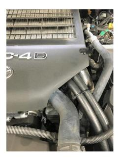
Step 16, Refit radiator guard and intercooler guard. Ensure hoses do not rub on intercooler guard. Install cable ties (item21) to prevent hoses from rubbing on sharp objects.
