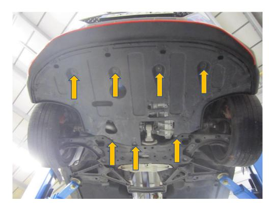
5. Both sides of the bumper now need to be parted from the vehicle, pull sharply at the top corner of the bumper so that it comes away from its locating clips as shown in the picture. With both sides now away from the body of the vehicle you will be able to pull the bumper off the front of the car.
