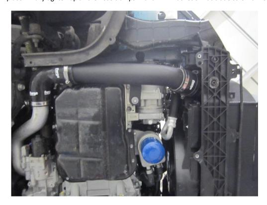
19. Now fit the near-side hose to the intercooler. This is also secured with 7mm hose clamps, the same as the off-side hoses.
