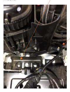
Step 8: Extend harness that plugs into bottom of Positive battery terminal by 300mm.
