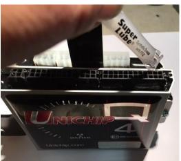
Step 11: Refit ECU Cover plate and mount Unichip Q4 and PD6 Driver to ECU cover plate.
