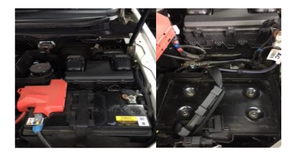
Step 2: Remove 2 Plugs from top of fuse box and remove power cable.
