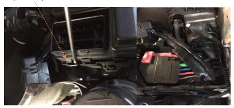
Step 4: Remove Fuse box base by unclipping loom and removing bolts holding it down.
