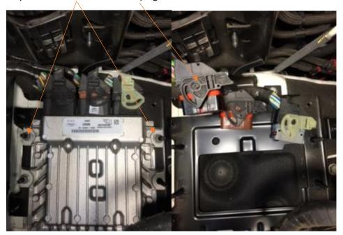
Step 7: Unbolt Fuel filter mount and re-route fuel filter wiring harness to back off car. Refit Fuel filter mount.
