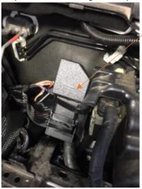
Step 13: Reassemble fuse box and battery in reverse order.
