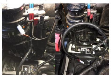
Step 9: Fit Unichip Plug and Play harness into Factory ECU and refit ECU.
