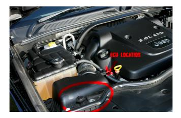
4. Remove the two plugs from the factory ecu by lifting the levers and sliding the tabs back (do not force)
