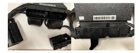
7. Connect Unichip harness plugs to factory ECU
