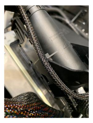
8. Connect factory ECU plugs into Unichip block
