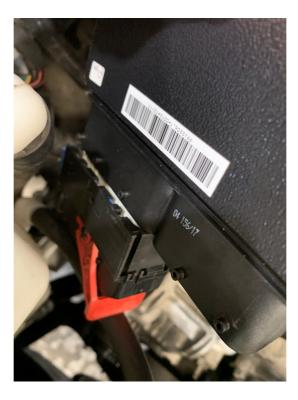
9. Plug Unichip harness into Unichip module
