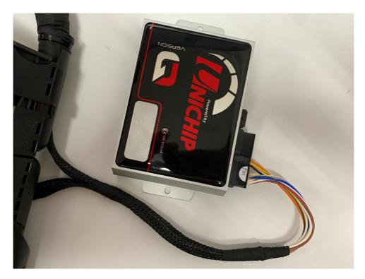
Secure unichip block to ECU with supplied Velcro.
