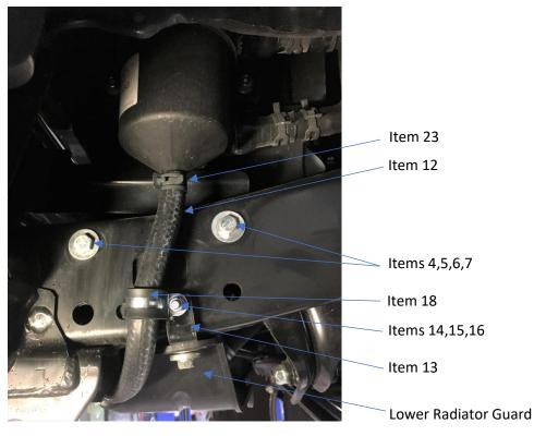
Step7: Install Provent assembly from the bottom of vehicle until Bracket lines up with holes in Chassis Rail. Install 8mmx70mm Bolts with 8mm Body Washers (Items 4,6) through chassis rail and Provent bracket. Install 8mm Flat washer and 8mm Nyloc nuts (items 5,7) and tighten as required.
