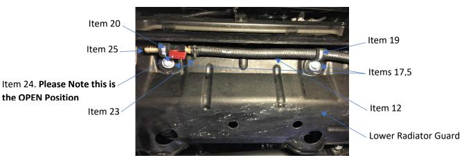
Step11: Run Drain hose around the front of vehicle.
