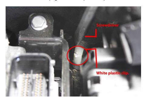
9. Run rear ECU plug behind ECU against firewall.
