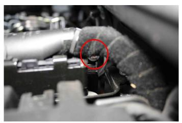
3. Using a centre punch and hammer hit front side of sheer off bolts, until they slightly turn.
