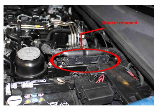
6. Unplug ECU plug by sliding locks back with a flat screw driver and unplug both ECU harness plugs.
