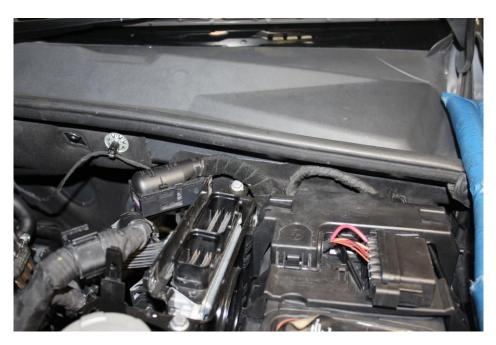
7. Fit plug and play harness to ECU factory loom.
