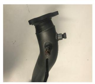
On the vehicles not fitted with a DPF use the supplied plugs to blank <u>all</u> ports on the Unichip dump pipes.
