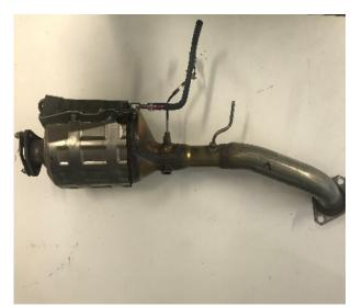
Fit both of these sensors and the provided blanking plug to the Unichip turbo dump pipes (DPF model only).
