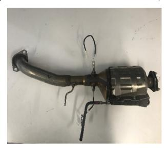
Remove the highest EGT sensors closest to the turbo and the oxygen sensors on both sides (DPF model only).
