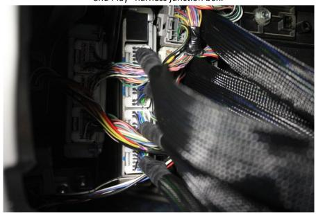
6. Fit the three Unichip Q4 Loom plugs to the Unichip Q4.
