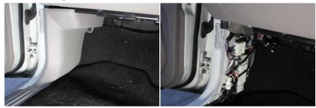
5. Remove Glove box, by lowering and unclipping. Remove black plastic glove box cover 5 screws and 2 body clips.
