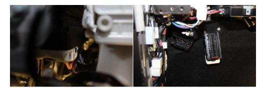
12. Connect small PNP plug first, fit up behind E.C.U against fire wall and fit plug to E.C.U.
