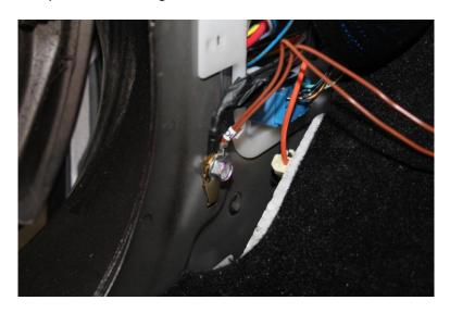
15. Measure 25mm deep x 100mm long from back of kick panel trim and remove material to clear PNP plug.
