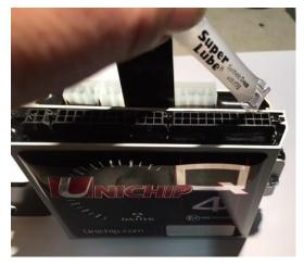
Step 11: Refit ECU Cover plate and mount Unichip Q4 and PD6 Driver to ECU cover plate.
