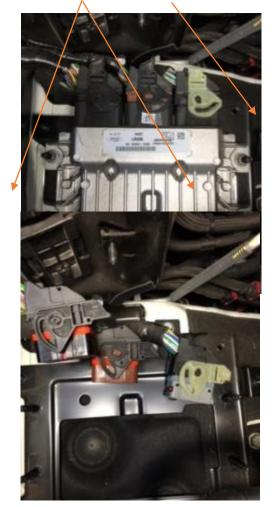
Step 7: Unbolt Fuel filter mount and re-route fuel filter wiring harness to back off car. Refit Fuel filter mount.
