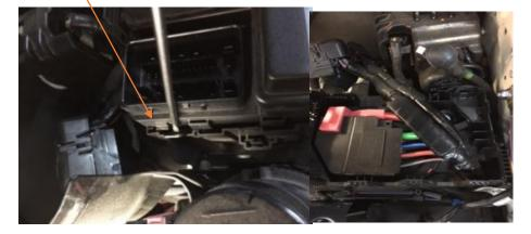
Step 4: Remove Fuse box base by unclipping loom and removing bolts holding it down.
