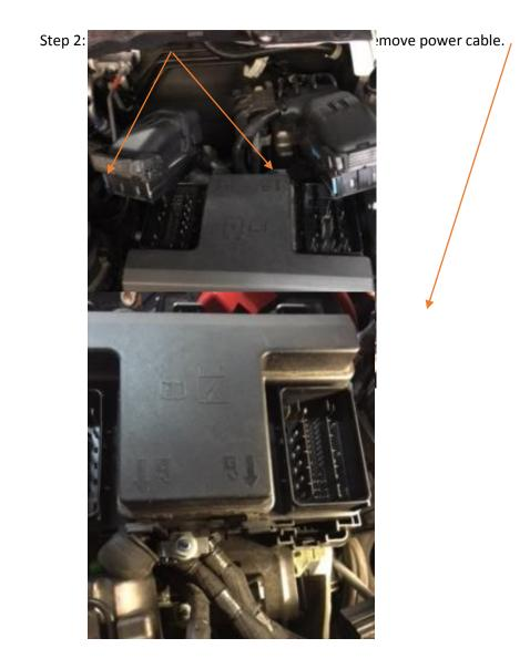
Step 3: Unclip Fuse box from base and remove.
