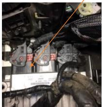
Step 10: Mount Unichip Q4 and PD6 Driver to bracket and apply Super Lube (dielectric grease) to terminals.
