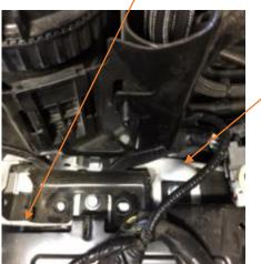
Step 8: Extend harness that plugs into bottom of Positive battery terminal by 300mm.
