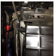
Step 6: Unbolt ECU and remove plugs. Remove ECU from vehicle.
