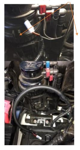
Step 9: Fit Unichip Plug and Play harness into Factory ECU and refit ECU.
