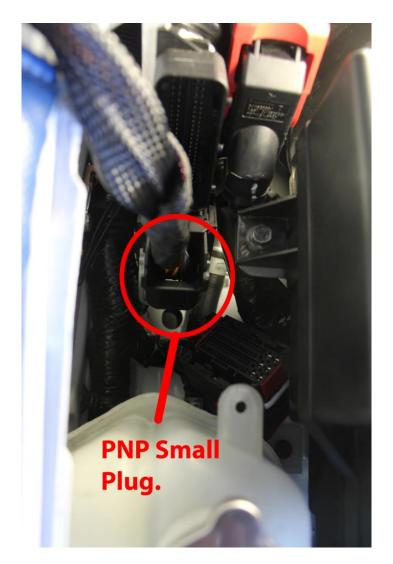
5. Plug Unichip PNP small plug harness into factory ECU. Plug small factory plug into Unichip PNP harness.
