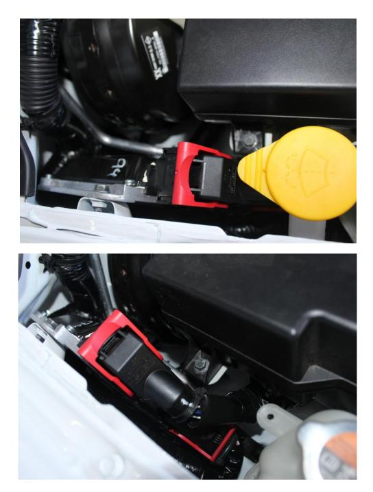
2. Remove windscreen washer filler, in front of E.C.U. (Right hand rear of engine bay).
