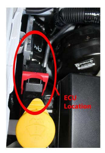
3. Locate ECU (Right hand rear of engine bay) and unclip Red ECU tabs, on both large and small ECU Connectors.
