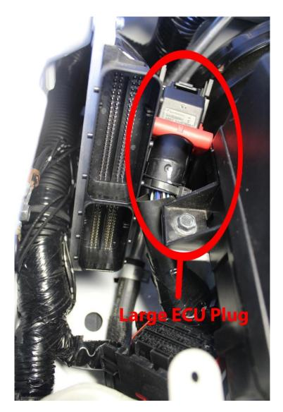
4. Feed Large ECU plug past Relay box towards rear of vehicle.
