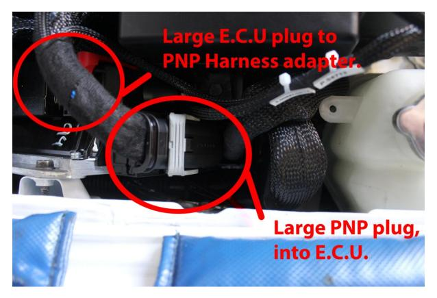
6. Plug Big Plug Unichip PNP Harness into factory ECU. Plug factory Big plug to PNP harness.
