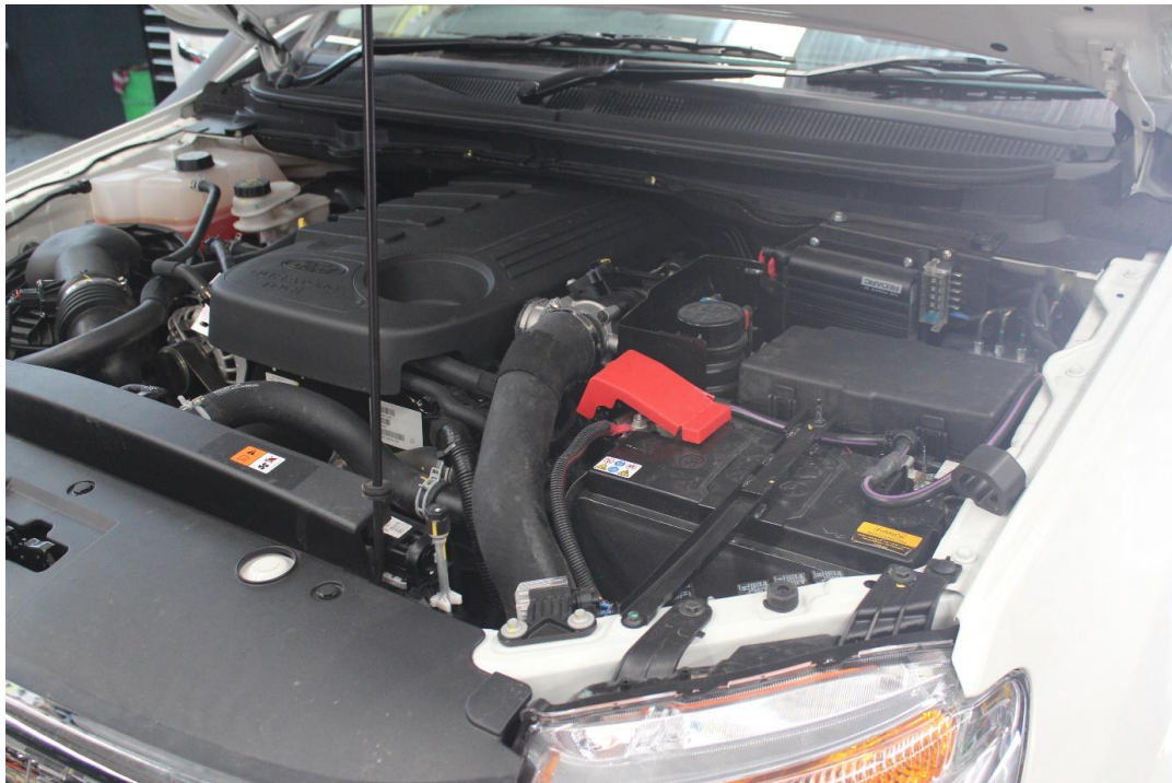
Step 12: Refit Battery ( positive terminal first )
