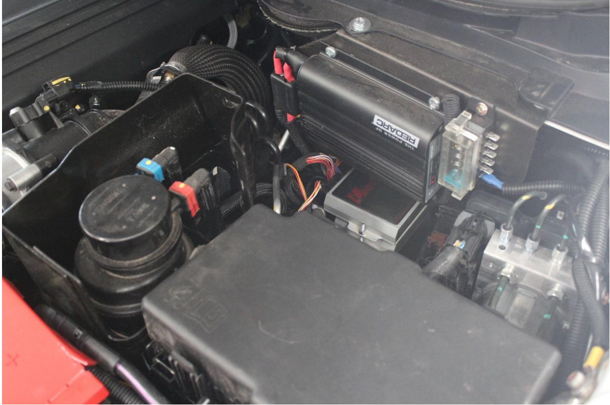
Step 12: Refit Battery ( positive terminal first )
