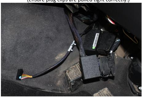
5. Fit plug and play harness to factory E.C.U. (Make sure plugs are square and horizontal to ECU when installing. DO NOT FORCE PLUGS.)
